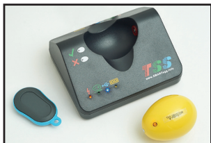
Egg damage testing (SMARTegg)
